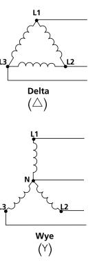
Since the difference between Delta and Wye is whether or not there is a neutral, many data centers are wired for Wye and use whips terminated with Wye receptacles such as NEMA L21-30R. This means the data center can use Wye PDUs which support 120V/208V or use Delta PDUs which support only 208V without needing to change the data center wiring.
