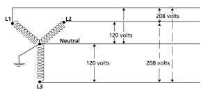
A Delta PDU would use a NEMA L21-30P (the mating Wye plug), but would not use a neutral inside the PDU. This is a perfectly acceptable practice. For example, a data center could deploy Delta PDUs to racks where there is only a need for 208V and Wye PDUs to racks where there is a need for both 120V and 208V.
